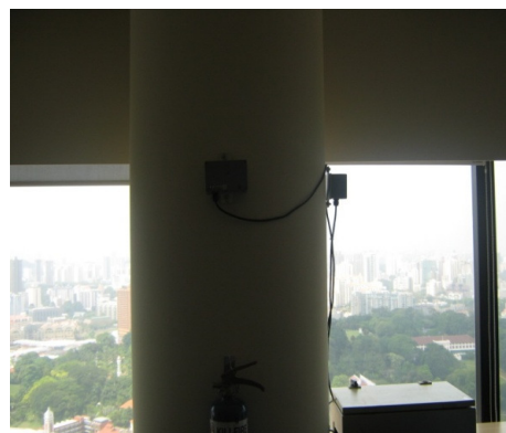
EL Tiltmeter installed on columns at client's office
