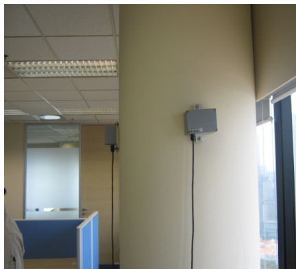
EL Tiltmeter installed on columns at client's office
